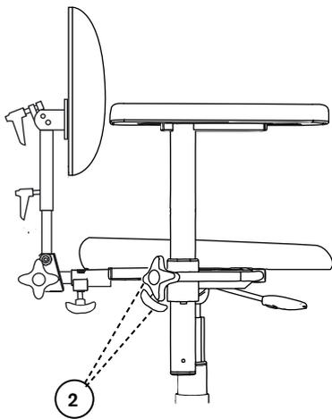
Loosen the regulators for the armrest (2). Set the desired level in height and width. Tighten all regulators (2).
